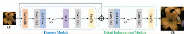
Figure 3. The overall structure of the RawRTSR-L network: 0.311M parameters and running at 4.44 ms on the A100 GPU.
