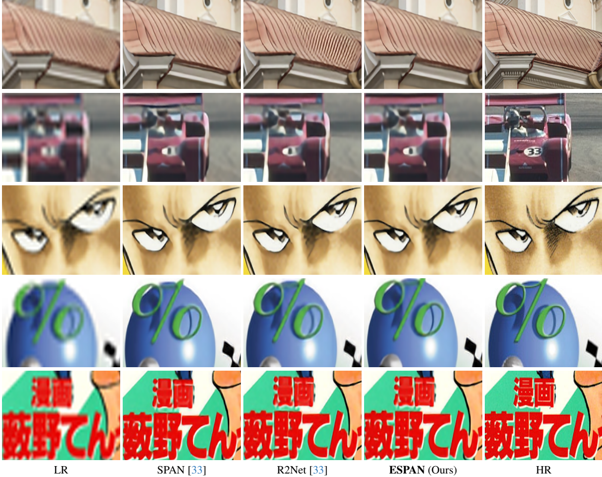
Figure 4. Visual comparison of ESPAN with other top ranking methods of the NTIRE 2024 ESR Challenge for the \times 4 super-resolution (SR) task on the public datasets.
