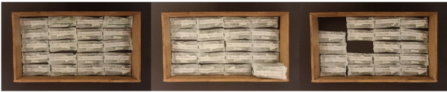
Figure 3. Defects in Pile of Packets sub-dataset - top row(left to right) :Normal, overload, under-load;
