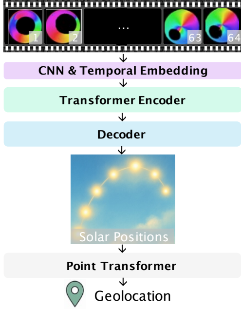
Figure 5. Model. A sequence of AoP frames and temporal data are embedded and processed by a transformer encoder to summarize the sequence. The input and the summary token are decoded by an MLP head to predict the solar-elevation curve. The estimated curve and temporal context are treated as a “point cloud” and fed to a point transformer, which regresses the geographical coordinates (\phi, \lambda) of the camera.
