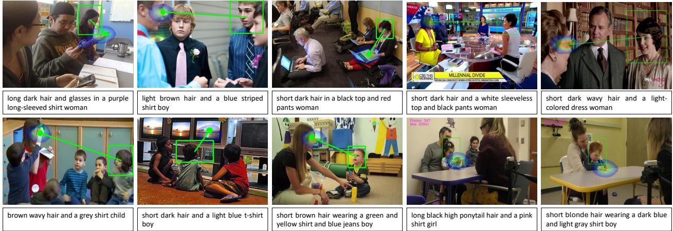
Figure 4. Visualization of GazeAnywhere’s gaze target estimation results from several datasets. The input is the text prompt (shown in the black box) describing only the subject person’s appearance and the image. GazeAnywhere detect the subject’s head and track the gaze target. More qualitative comparison is shown in the appendix.
