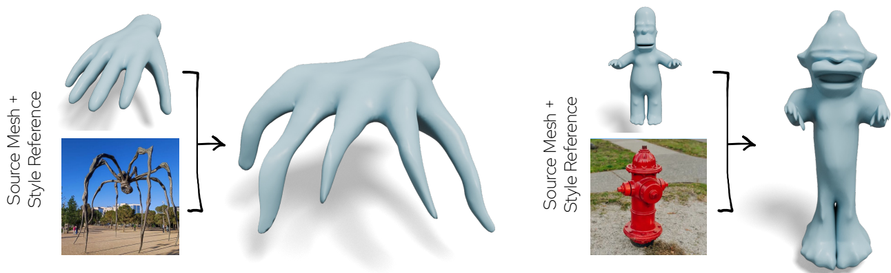
Figure 1. Our method enables stylization of 3D meshes driven by image style references. The target stylized meshes retain the coarse structure and semantics of the input mesh while incorporating internal geometry derived from the style reference.
