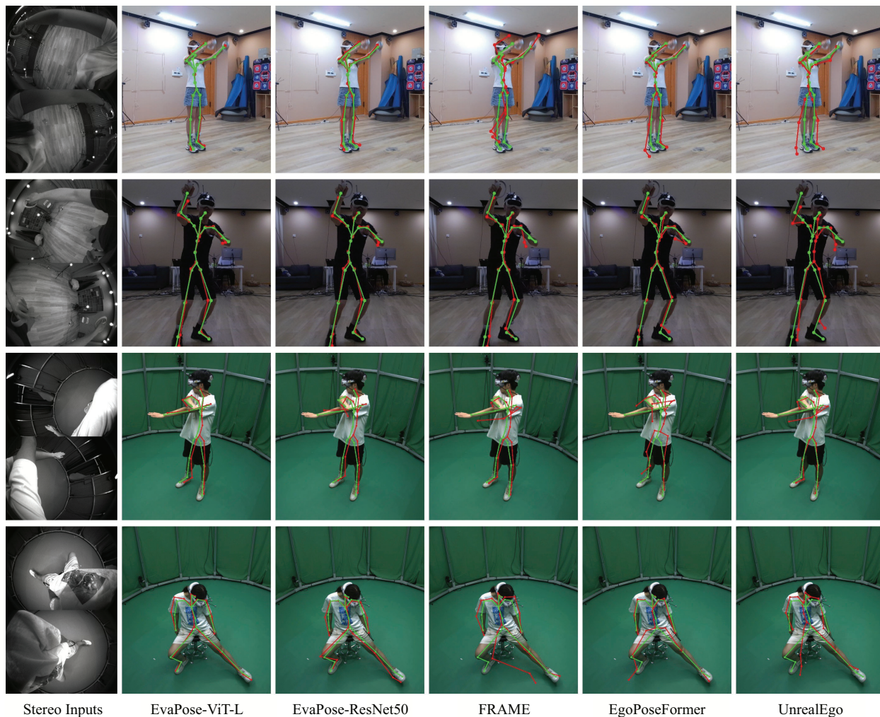
Figure 3. Qualitative comparisons on both EMHI (the first two rows) and Eva-3M (the last two rows) datasets. For better illustration, the predicted (red) and ground-truth (green) 3D poses are re-projected onto external reference views which are not used for pose estimation.
