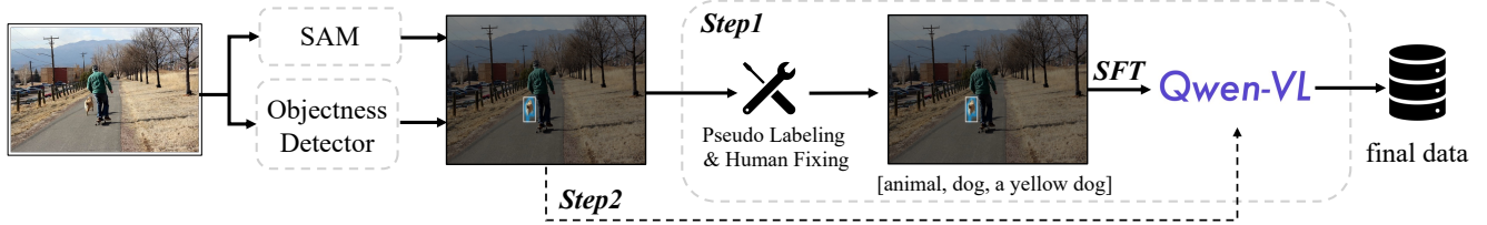
Figure 2. The proposed data engine. We first use an objectness detector to detect all regions of interest along with masks produced by SAM. Then, an LMM is used to generate multi-granularity and instance-specific labels for each object. The LMM is finetuned by us to ensure high-quality labeling and structural output.
