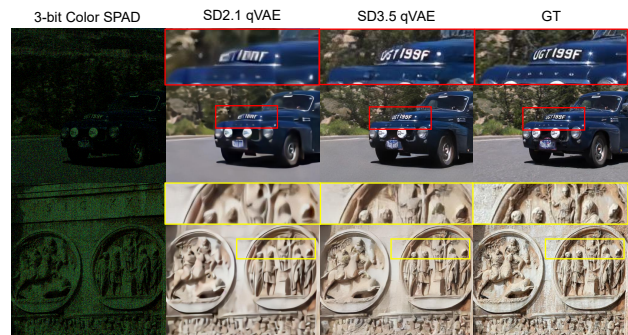
Figure 7. SD3.5’s VAE solves the text problem [4, 5]. SD3.5 [14] uses a 4× larger latent space than SD2.1. This yields sharper high-frequency details and legible text drawing capabilities.
