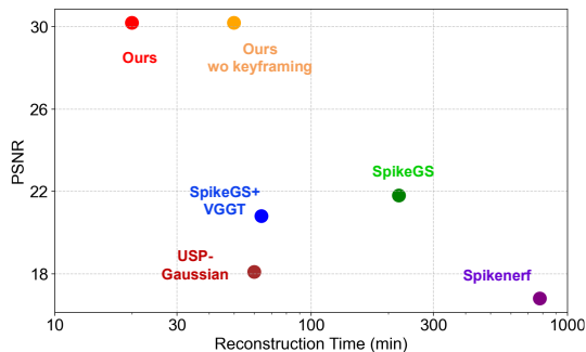
Figure 8. Comparison of rendering quality and efficiency with prior spike-based 3D reconstruction methods.
