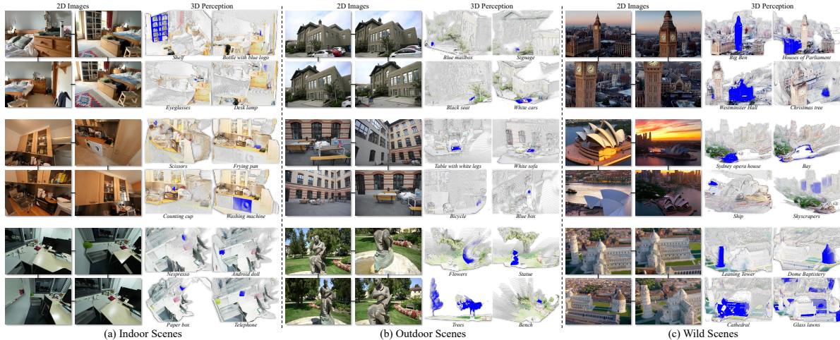
Figure 1. Examples of Perception-Efficient 3D Reconstruction. Our framework reconstructs 3D semantic scenes from unposed RGB images and supports open-vocabulary interaction, without any training or per-scene optimization. It is efficient in two critical ways: (1) Input efficiency : no depth maps or camera parameters are needed; (2) Inference efficiency : significant speed gains on semantic reconstruction compared to prior pipelines. These properties make PE3R practical for real-world deployment in large-scale and time-sensitive scenarios.
