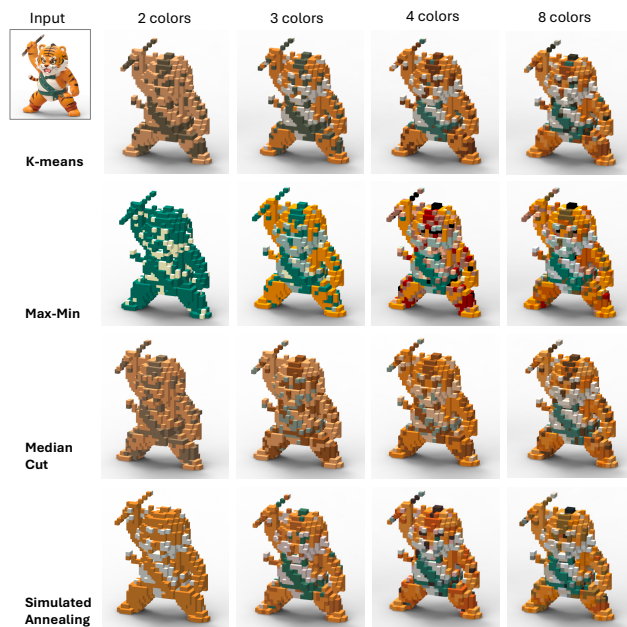
Figure 7. Effect of Palette Selection and Color Count. Each row corresponds to a different palette extraction method: K-means, Max-Min, Median Cut, and Simulated Annealing. Each column shows increasing color counts (2, 3, 4, 8). Each method produces unique color clustering effects.
