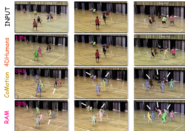
Figure 1. RAM performs online 3D motion reconstruction from monocular video via semantic, motion-aware tracking and occlusion-robust prediction. Unlike prior methods that rely on frame-wise regression and queue-based identity matching, which are often unstable under fast motion and occlusions, RAM maintains consistent identity and accurate reconstruction, while achieving real-time performance that is 2–3× faster than previous approaches. Arrows highlight key differences.
