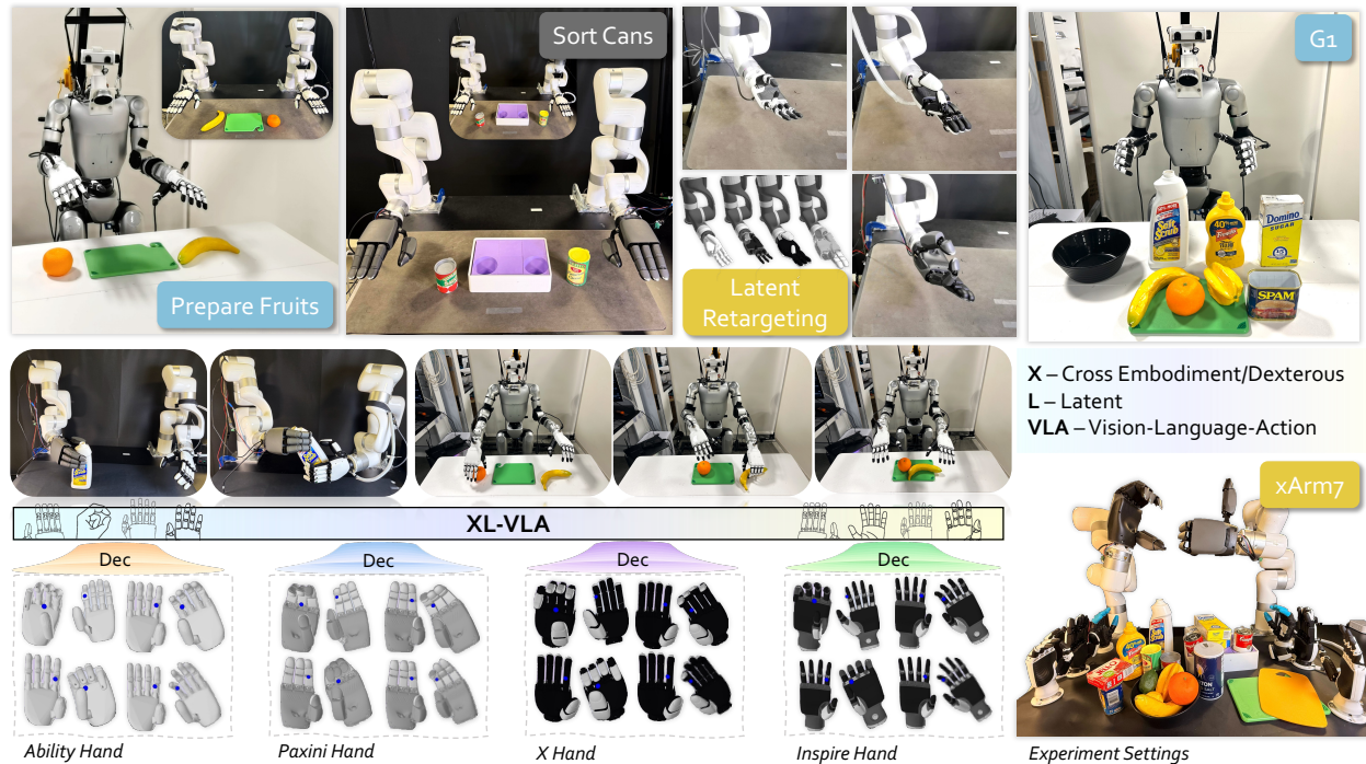
Figure 1. Overview. XL-VLA enables direct decoding of a single latent action into multiple dexterous hand embodiments. Shown above, an action prediction can be instantiated on the Ability hand, Paxini DexH13 hand, X-Hand1, and Inspire hand for language-guided manipulation. We show our experiment settings on the right figure with collected objects and DexHands.
