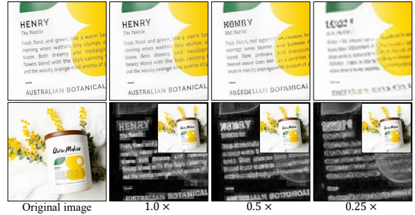
Figure 4. Example of one-step denoising distortions. For each distortion level, pixel-wise variance maps are computed over 10 degraded samples. Insets show example outputs, with distortions concentrated in high-frequency regions.
