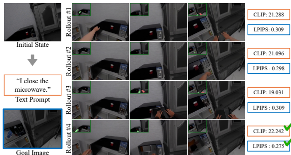
Figure 7. Action evaluation. DWM simulates multiple candidate actions and ranks them based on goal alignment.
