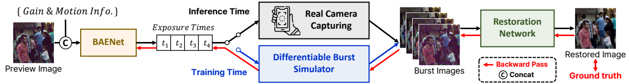
Figure 1. Overview of our pipeline. BAENet predicts the exposure times of each burst image from a preview image. Differentiable Burst Simulator generates burst images according to the exposure times. The restoration network then reconstructs a high-quality image from them. During inference, the simulator is removed, and the restoration network processes real burst images captured by our camera system.
