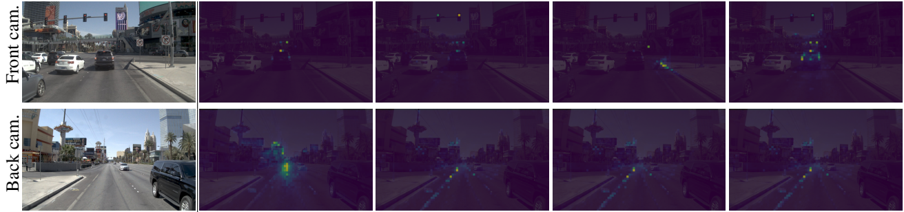
Figure 4. Attention maps of scene tokens. From the final attention layer, front-camera tokens specialize to distinct regions (traffic light, lead vehicle, road edges), while back-camera tokens largely collapse to the same features, aside from a single distinct token.
