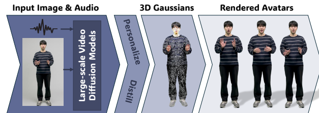
Figure 1. Overview of our personalized Audio -driven whole-body talking Avatars (AudioAvatar) : End-to-end framework that distills large video diffusion models to generate expressive, synchronized talking avatars from a single image.
