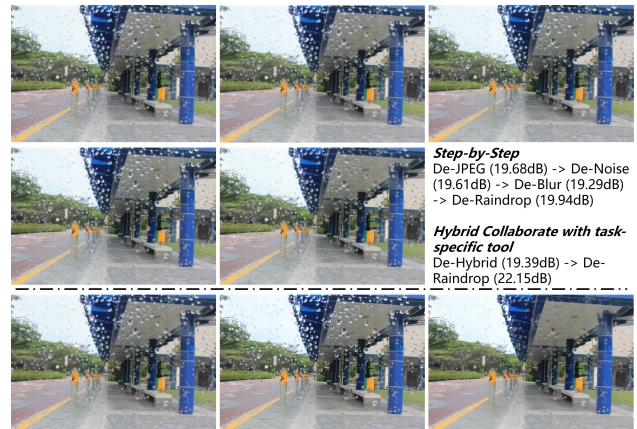
Figure 5. A case study on complex degradation removal. The image is corrupted by “Raindrop + Blur + Noise + JPEG”. Upper: step-by-step distortion removal. Bottom: tools invoked by HybridAgent: De-hybrid + De-raindrop.
