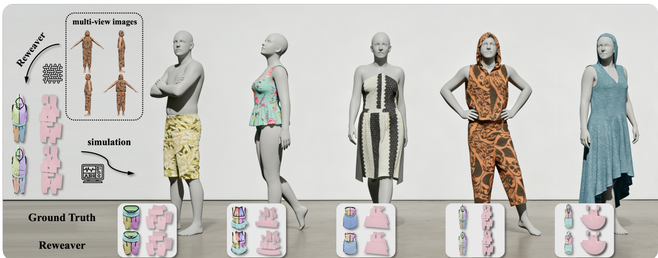
Figure 1. ReWeaver . From as few as four input views, ReWeaver reconstructs high-precision sewing patterns with complex topology together with their corresponding 3D geometry. The method outputs a unified 2D–3D garment representation, where each panel and edge is explicitly linked to its associated 3D points. This enables faithful, simulation-ready garment assets to be recovered from ordinary and sparse-view photographs without a controlled capture setup. The reconstructed garment geometry and topology is precisely aligned with the input images and can be used for 3D structural perception.
