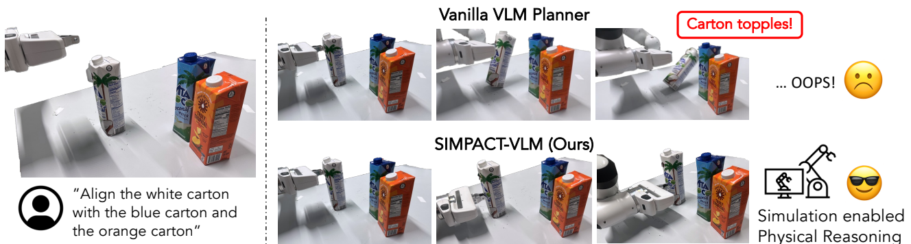
Figure 1. Simulation-Enabled VLM Action Planning. Given a single RGB-D image and a language task description ( left ), our method efficiently constructs a physics simulator that enables test-time VLM reasoning with physical grounding. This physically grounded reasoning allows the robot to succeed in fine-grained manipulation tasks ( bottom ), outperforming a vanilla VLM planner ( top ) that lacks awareness of physical dynamics.
