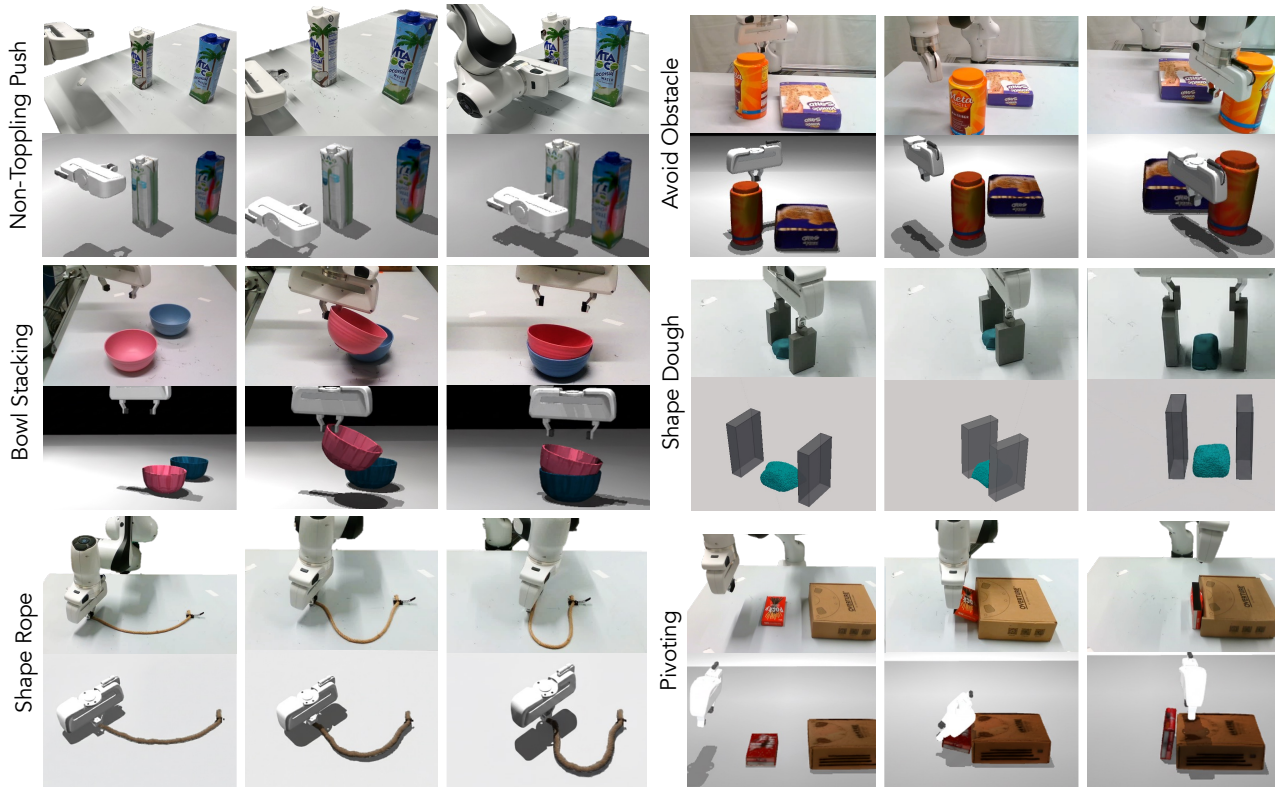
Figure 5. Qualitative results. The figure shows the initial state, execution progress, and final state for six tasks in both the real world (top) and the simulation (bottom). By leveraging VLM’s powerful generalization, rendered simulation images can guide VLM’s test-time reasoning for action planning despite the visual sim2real gap. Fig. 10 shows the results of the remaining task.
