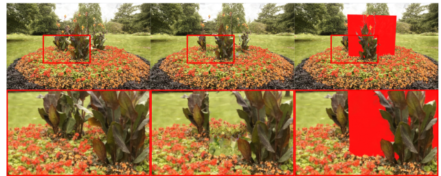
Figure 8. Editing demonstration. Left: Original. Middle: Delete the same cube. Right: Add a red cube. We perform these edits by adding points to the surface of the edit volume, re-triangulating the scene, then modifying the cell values.
