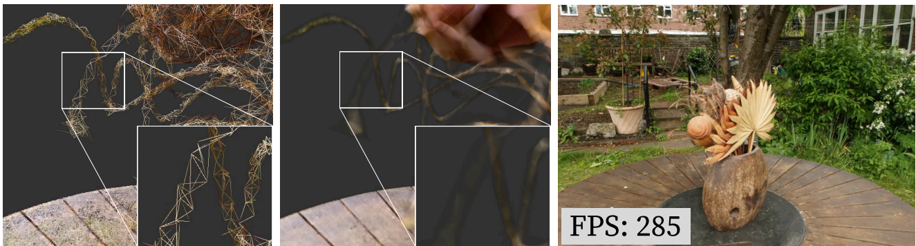
Figure 1. A radiance mesh parameterizes a radiance field using the tetrahedra produced by a Delaunay triangulation of a set of points, where each tetrahedron has a constant density and a linearly-varying color. This representation allows us to use traditional mesh processing (left) while still enabling semi-transparent rendering (middle), which allows our model to be rendered using a hardware triangle rasterizer very quickly on a wide variety of platforms (right). See the supplement for an interactive web demo.
