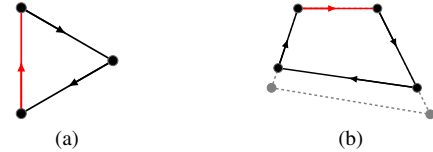
Figure 2. Toy examples of graphs in \mathbb{R}^2 with input directions (arrows) depicted as edges that form loops. The output we seek is the set of node values satisfying the input directions. When we fix the red edge’s scale, (a) has only one solution for node values (black), while (b) has infinite solutions (another solution in gray by scaling the black edges to gray ones independent of the red edge). The independent scaling in (b) occurs with any set of four directions forming loops; thus, this issue is due to its topology. Hence, (a) is a generically parallel rigid graph in \mathbb{R}^2 while (b) is not.
