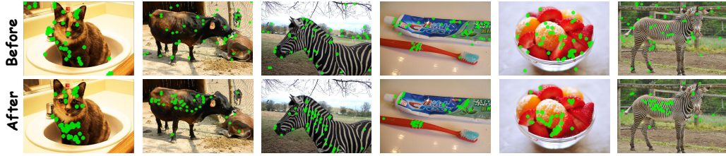
Figure 5. Effect of the Centerness-Guided Query Selection. Visualization of query selection before and after applying the Centerness-Guided Query Selection (CG-QS) module. Each pair of heatmaps (top: before, bottom: after) corresponds to the same image. After applying the CG-QS module, the model tends to select queries near object centers, thereby generating more accurate proposals.
