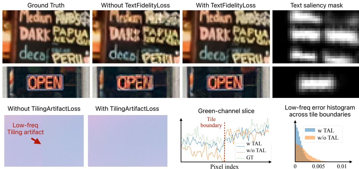
Figure 7. Ablations on artifact-specific mitigation strategies. All images are encoded at a BPP 0.20. Top: Perceptual training leads to distortions in text, while adding the TextFidelityLoss enhances its fidelity. On the right we show the text saliency masks. Bottom: TilingArtifactLoss (TAL) mitigates color mismatch artifacts at tile boundaries (please zoom-in to better visualize). In the middle we show a slice in the green channel across the tile boundary, where reconstruction without TAL exhibits discontinuity. On the right we show a histogram of error around tile boundaries over the CLIC 2020 Professional Validation Set, which is significantly reduced by TAL.
