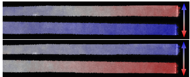
Figure 1. Recovered displacement of a vibrating tuning fork. We unwrap the phase to recover per-pixel displacement. The top and the bottom prong move in equal and opposite directions, showing the fundamental resonance mode. The tip of the tuning fork is on the right-hand side of the image.
