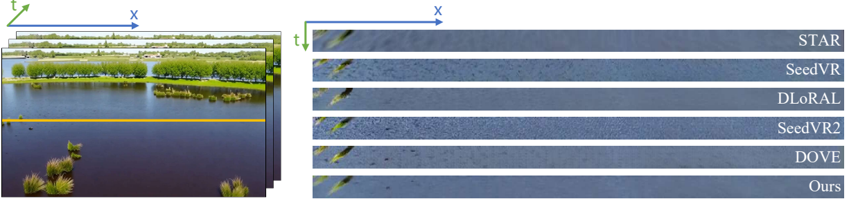
Figure 4. Comparison of temporal profile that tracks variation of the pixels in a spatial row (highlighted by the yellow line). The width of the temporal profile equals to the video width, and the height is the number of frames of generated high-quality video.
