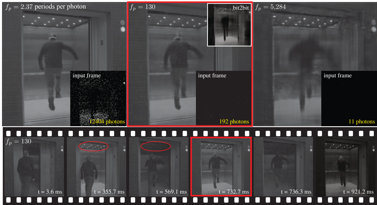
Figure 1. Videography in the inter-photon-limited regime. Our method reconstructs high-quality video from binary photon detections or timestamp data when scene intensity fluctuates faster than photon arrivals. We characterize this regime using the inter-photon frequency f_p in periods per photon, which directly couples the speed of photon arrivals and scene variations in a timescale-invariant manner. Bottom: Our method reconstructs both periodic (light flicker) and non-periodic scene variations (elevator door, human motion) simultaneously.
