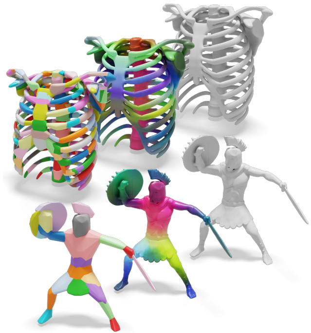
Figure 1. Our method takes an input shape ( top ), infers features from an open-world model learned with our new self-supervised geometric loss ( middle ), and clusters those features to fit the shape with a collection of tight convex bounding proxies ( bottom ).
