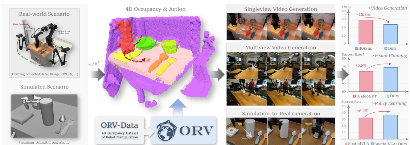
Figure 1. We condition robot video generation on 4D semantic occupancy sequences and 7-DoF actions collected from real and simulated environments (through methods \pi and \pi' ). This occupancy-centric conditioning enables faithful, controllable synthesis of single-view, multi-view, and sim-to-real manipulation videos. We also introduce ORV-Data, a curated 4D occupancy dataset for robot manipulation. Across benchmarks and downstream tasks, ORV improves video quality and control alignment, boosting visual planning and policy learning.
