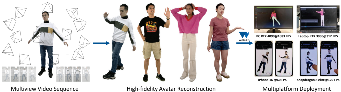
Figure 1. Our method creates high-fidelity human avatars from multi-view video. The avatar can run on multiple platforms, including desktop PCs and mobile devices with ultra-fast rendering speed (1683 FPS on an RTX 4090 GPU and 120 FPS on mobile devices).
