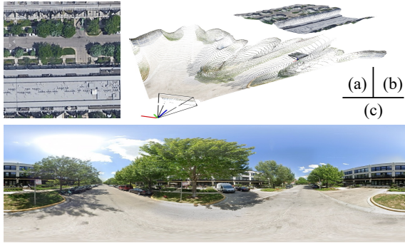
Figure 1. Illustration of directly using VGGT on satellite (a) and ground (c) images, leading to incorrect reconstructed shown in (b).
