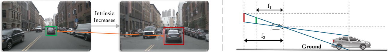
Figure 2. Impact of intrinsic variation on image appearance. Left: The two images show the same object in the same 3D position but captured with different intrinsics. As the focal length increases, the object appears larger and the FoV is smaller. Right: Schematic illustration of how intrinsic variations affect object appearance.
