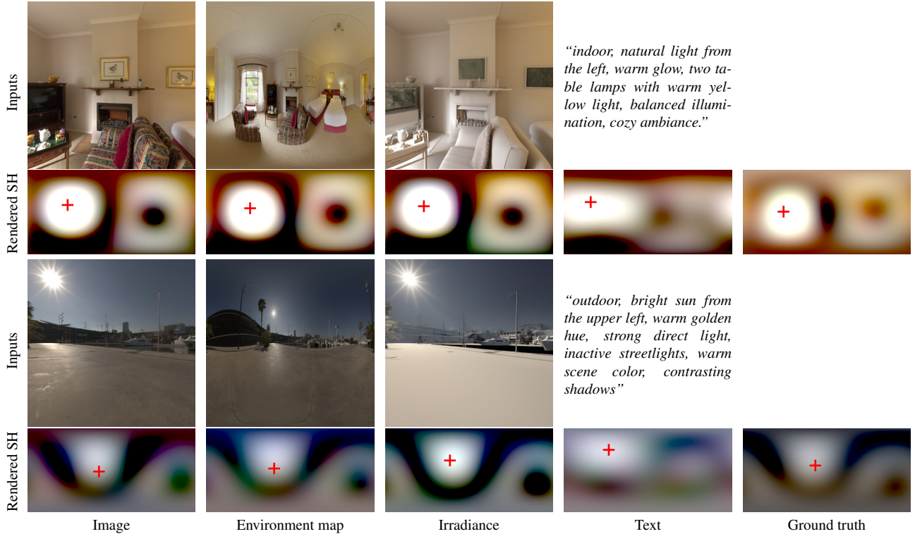
Figure 6. We visualize the SH coefficients extracted by our SH head (see Fig. 3) from the UNILIGHT embeddings of the input modalities (rows 1 and 3). We render the predicted SH to an environment map (rows 2 and 4) and visualize the dominant light direction as a red cross. Note how both the reconstructed environment maps and the dominant light directions align across modalities as well as with the reference, indicating that they indeed have similar latent embeddings.
