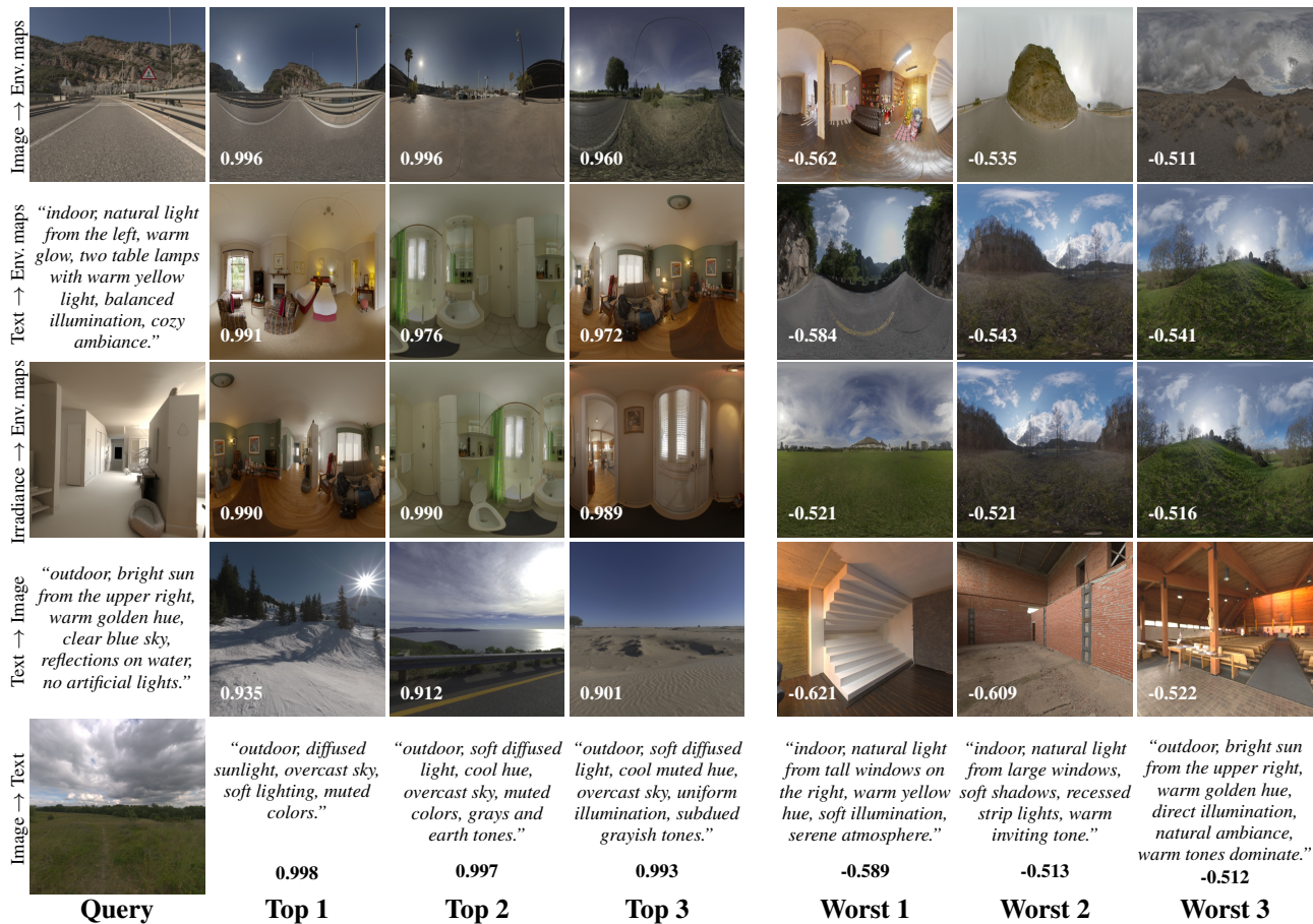
Figure 8. Top-three retrieval comparisons across different modalities in the rows. For example, the first row embeds an image and retrieves environment maps, using the image’s UNILIGHT embedding as a query. Columns show the three best and worst matches. The inset values are the cosine similarities between query and result embeddings.
