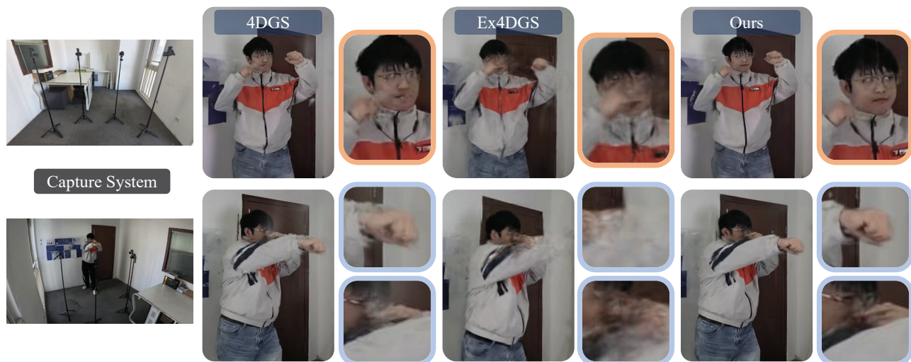
Figure 1. Left: Our capture system records dynamic scenes using only four cameras. Right: Dynamic novel views rendered from the reconstructed 4D representations produced by 4DGS, Ex4DGS, and our method.
