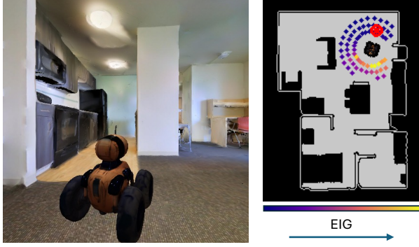
Figure 5. Generation of candidate viewpoints for Object Mapping Mode. When the EKF becomes confident, Paparazzo switches from tracking to mapping and evaluates a set of candidate viewpoints \mathcal{V} distributed around the object. The expected information gain (EIG) of each pose, computed using the FisherRF criterion, is visualized here with a color gradient: darker tones correspond to low informativeness, while brighter tones highlight more informative poses for reconstructing the object.
