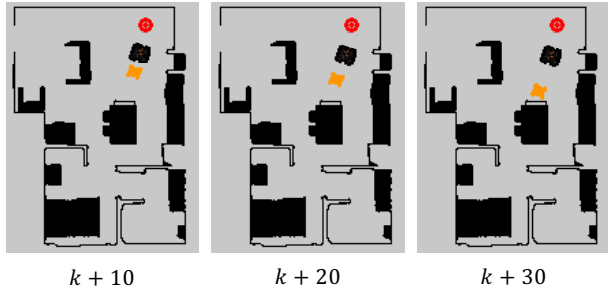
Figure 6. EKF-based prediction of future object poses. The EKF predicts the object pose, denoted in orange, over the next N_h steps. The figure shows three examples at steps k+10 , k+20 , and k+30 . These predicted poses are then used to propagate all candidate viewpoints \mathcal{V} into the future, producing a set of |\mathcal{V}| \times N_h future-aligned viewpoints that are subsequently evaluated by the final cost function in Eq. (3).
