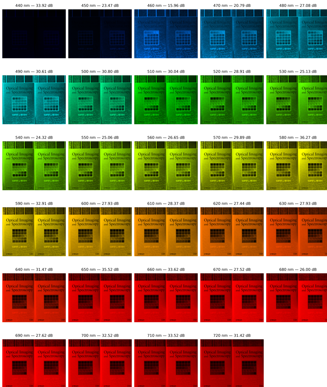
Figure S20. Full reconstruction of book scene. Per-channel images (left: ground truth, right: reconstruction). See per-channel labels for central wavelength and reconstruction PSNR.
