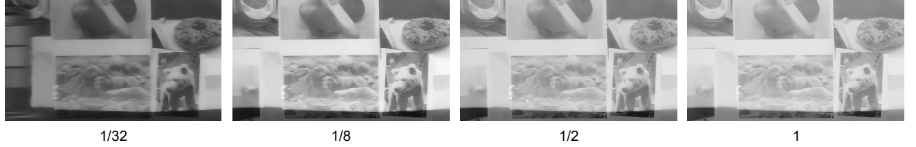
Figure 7. Reconstructed first frame comparisons with different aperture speeds. We compare 1/32, 1/8, 1/2, and the maximum speed. Please zoom in for more details.
