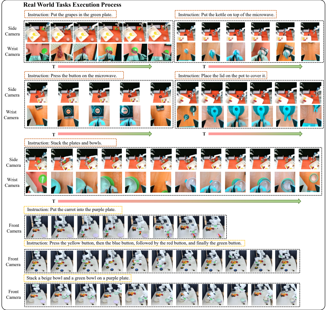
Figure 2. Visualization of Dobot and Franka Robots' Execution Processes in Real-World Environments. In the figure, the T-axis represents the time axis, indicating the duration from the start to the end of the task. Each demonstration shows the following elements: side and wrist camera views for the Dobot robot, and a single front view for the Franka robot.
