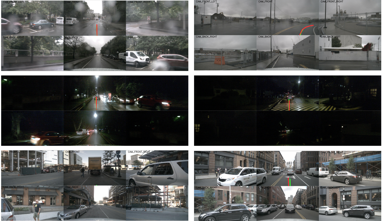
Figure 3. Qualitative results of HybridDriveVLA in diverse conditions. (Top) Navigating in cloudy and rainy weather. (Middle) Driving in a poorly lit environment at night. (Bottom) Driving in a dense urban area. HybridDriveVLA adapts by prioritizing safety, comfort, and progress. The optimal predicted trajectory is shown in red and the ground truth in green.
