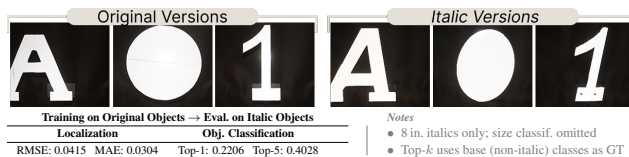
Figure 11. Generalization to modified object shapes. Top: italic-styled variants of three objects (A, 1, circle) captured at 8 in. Bottom: 1D CNN evaluation when trained on base objects and tested on italic variants. Performance is reasonable but below main paper baselines, as expected with shape/style distribution shift.
