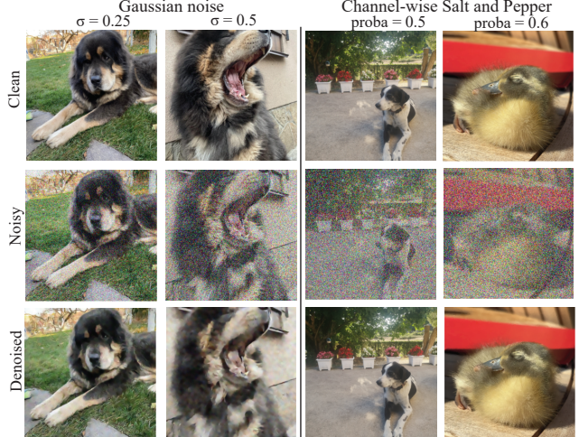
Figure 9. Image restoration using NAF. On the left two images we apply a gaussian noise. On the right we apply a channel-wise salt and pepper noise. NAF allows to restore very noisy images even on unseen noise range (rightmost image).
