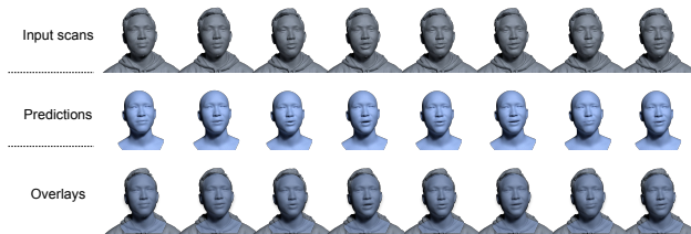
Figure 6. The CUBE scan encoder produces temporally smooth results for input scan sequences and can be used for performance registration. In this figure, we show the input scan, the prediction of our model and an overlay of the prediction on the input scan for a sequence of scans reconstructed from a facial performance of a subject. Note that the scans were processed independently for each frame.
