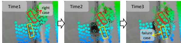
Figure 7. A failure case of a shaking toy caused by inaccurate event-camera depth estimation.
