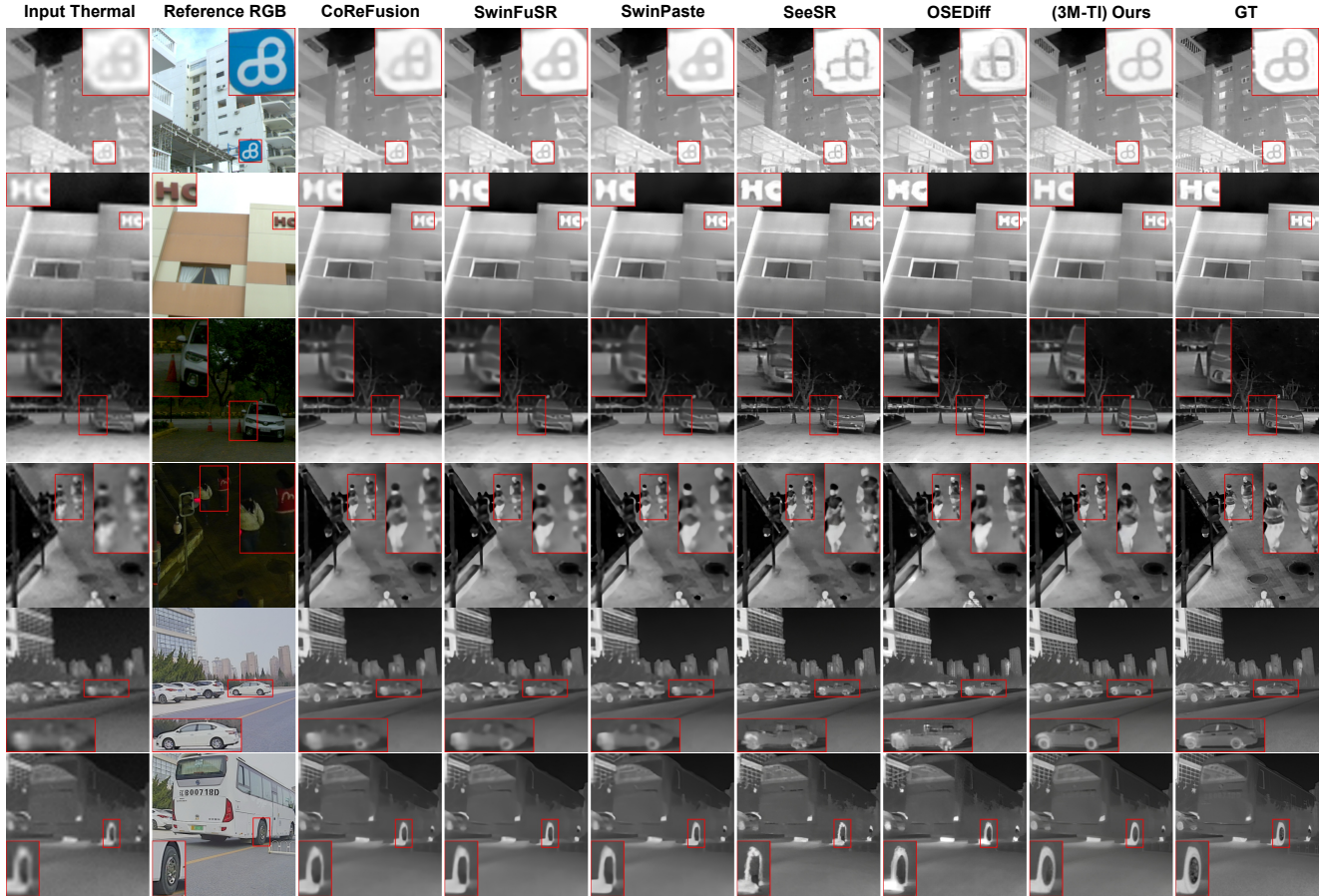
Figure S1. Qualitative comparison on our test set (zoom in for details). 3M-TI produces the most faithful and visually consistent results, delivering sharp structures and accurate thermal patterns that align closely with the GT. Representative examples include the sign (Row 1), English characters (Row 2), the traffic cone and car (Rows 3 and 5), and the pedestrians (Row 4).
