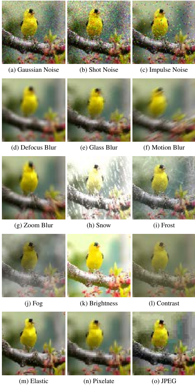
Figure 3. Illustration of ImageNet-C under five levels of severity. The dataset showcases 15 types of algorithmically generated corruptions across four categories: noise, blur, weather, and digital. Each corruption type is illustrated at five increasing levels of severity, demonstrating the progressive impact of these corruptions.
