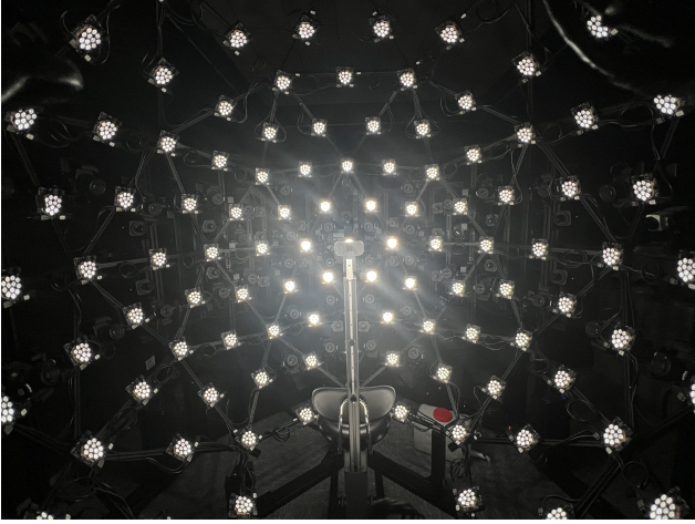
Figure A. Light stage. POLAR is captured using a calibrated light-stage setup that provides controlled illumination and high-fidelity appearance capture.
