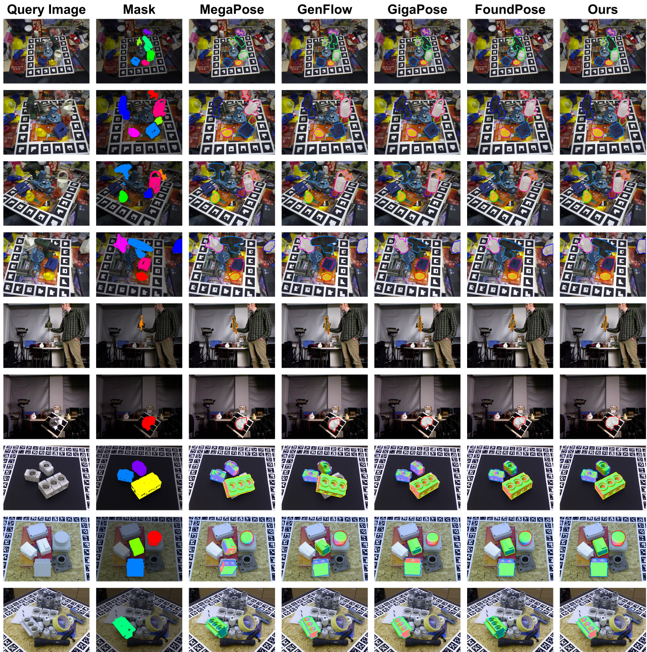
Figure 3. Visual comparison with other methods. From left to right: the query image for pose estimation, object masks with each object shown in a distinct color, and the projection results of different methods after applying the estimated poses to the 3D object models. The projected 3D models are outlined with borders matching the colors of their corresponding masks. The last three rows show samples from the T-LESS dataset [3]; since this dataset does not provide object textures, we display the rendered normal images of the objects for clearer visualization.
