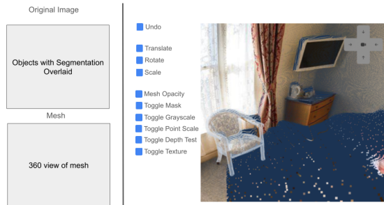
Figure 12. Stage 3 UI Sketch. The UI supports annotators in directly placing the object in the 2.5D pointcloud.
